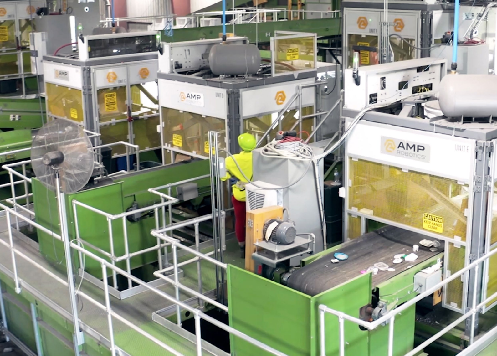
AMP Robotics sorteringsystem implementerat hos Single Stream Recyclers i Florida
